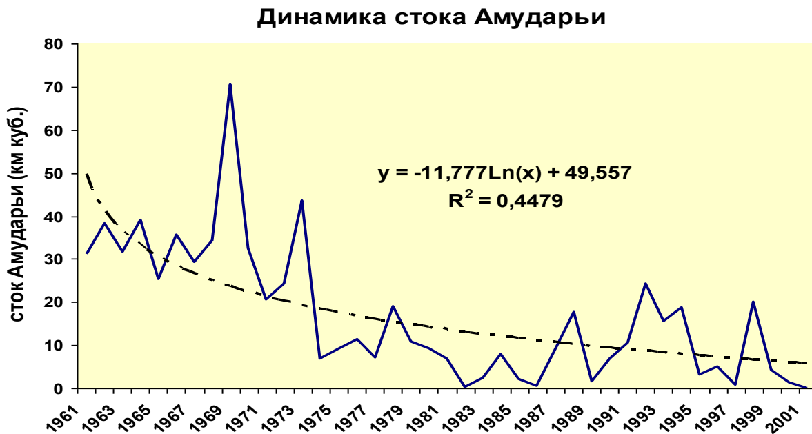
Pic. 1 Long-term dynamics of the Amu Darya runoff and its trend (dotted line)
